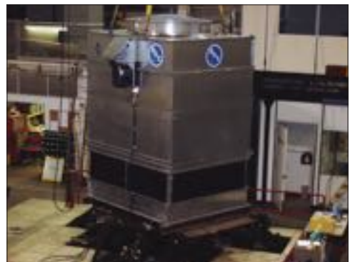
PT2 During Shake Table Testing
